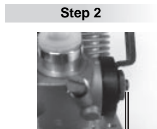
Low Speed Mixture: 1/16" of screw showing (1.5 mm) or 2 to 2 1/2 turns counter clockwise from clock.
